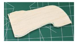
6 Here is my first piece with some scribe lines that show additional material that needs to be removed. Again, I use the Dremel tool for all the detailed removal. I cut out two pieces, one from the bottom of the opening and the other for the top; in most cases, they will be very close to the same size.
