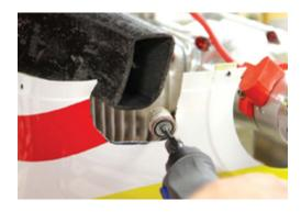
3 The cowl on this TOC Katana comes in two parts and allows me to work on the lower part while it is still attached to the aircraft. This makes my job of fitting the duct work much easier. I begin by enlarging the entry hole using the sanding drum on my Dremel tool. My Shop-Vac sucks up any dust created from the sanding drum and keeps the area clean.
