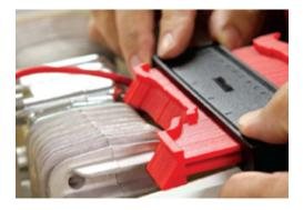
4 I start by using a pattern duplicating tool to make a rough outline of my engine head. I then transfer this outline to the 3/32 balsa wood. This pattern does not have to be exact and can also be created from cardboard or any other material you want to use.
