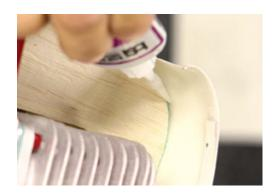
7 I now take both pieces and tack-glue them into place using BSI thick CA glue and placing two to three drops around the edge where the ducting contacts the cowl. Then I hit it with a quick spray of CA accelerator to hold my piece firmly in place. I repeat this process on the upper duct, or baffle, so it is also tacked in securely.
